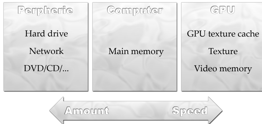
Figure 2. Hardware can be classified depending on a speed/amount ratio.
