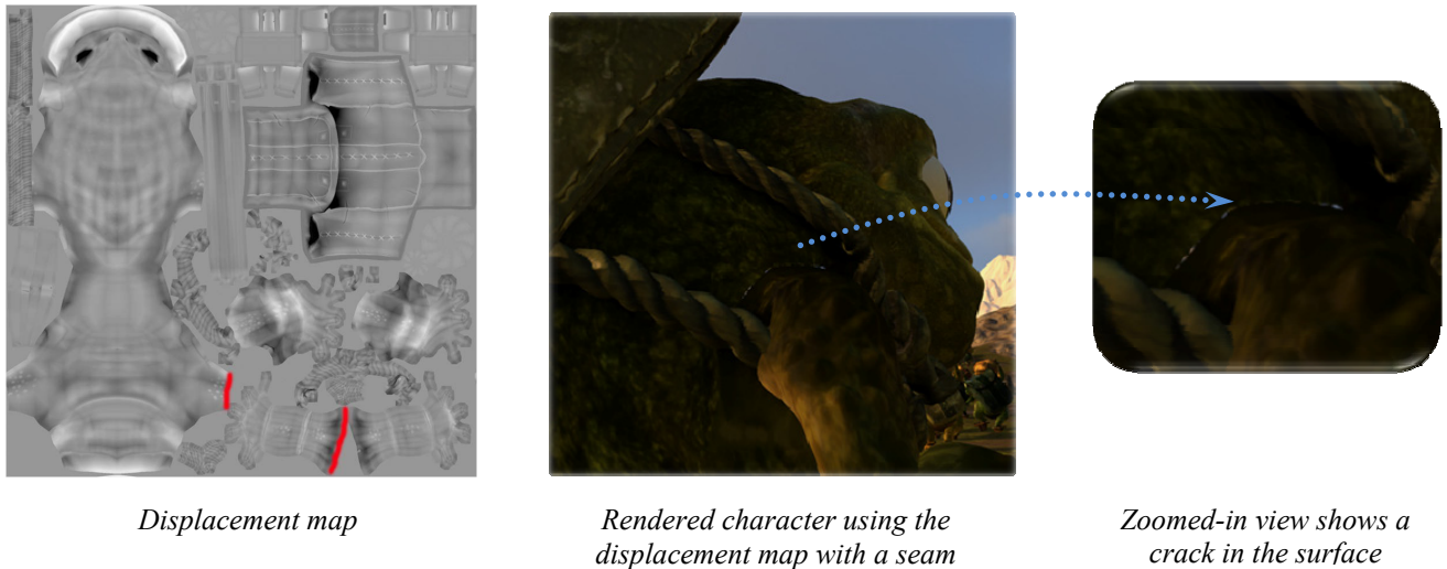
Figure 14. Example of a visible crack generated due to inconsistent values across the edges of displacement map for this character. On the left we highlighted the specific edges along the seam. Note that the adjacent edges for this seam do not have uniform parameterization.
